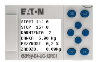
Ready! The feeder has loaded the settings we set and is in operating mode, which should be confirmed by the green LED on the housing.
